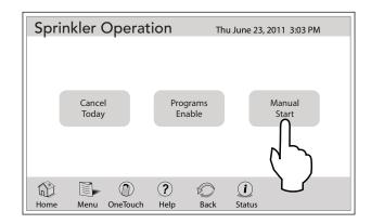
Continue on the screen shown below and click the desired PROGRAM # and click the START button. The program is started immediately and runs to completion unless interrupted by the user.
