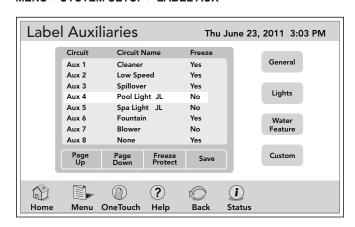
**NOTE** Please be aware that if the label NOT USED in the GENERAL LABEL menu is used on an AUX relay, the relay will not engage.
