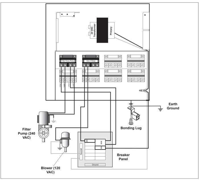
Figure 3. Standard Power Center - Bonding
