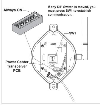
Figure 36. DIP Switch Settings at Power Center J-Box
