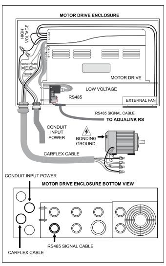
Figure 10. Wiring of the Jandy ePump<sup>™</sup> AC Variable Speed Pump to the Enclosure
