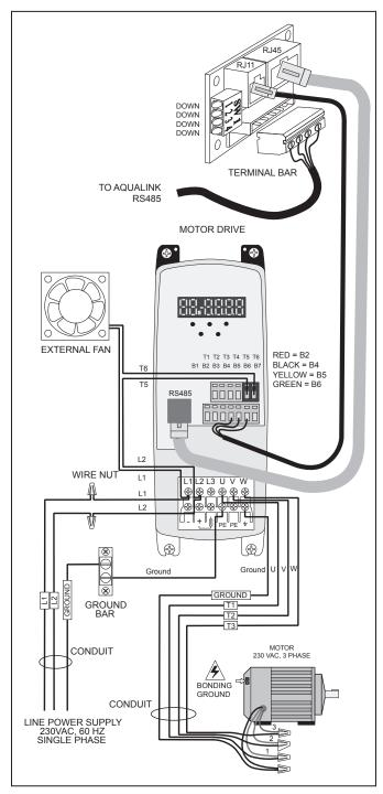
Figure 9. Wiring of the Jandy ePump<sup>™</sup> AC Variable Speed Pump to the Motor Drive
