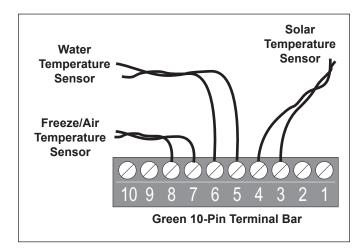
Figure 20. Temperature Sensor Wiring for a Pool/Spa Combination
