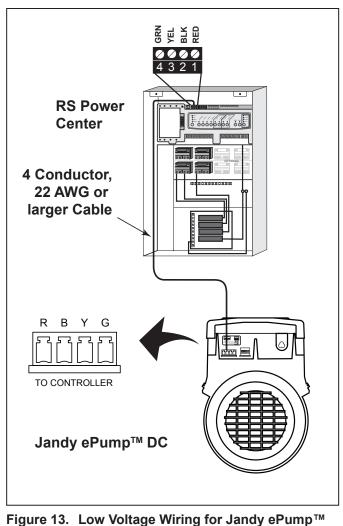
igure 13. Low Voltage Wiring for Jandy ePump™ DC
