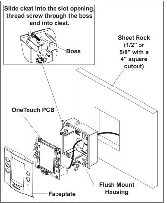
Figure 29. OneTouch™ Flush Mount Installation
