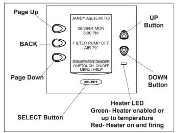
Figure 38. OneTouch<sup>™</sup> Control Panel Buttons
