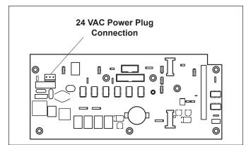
Figure 11. Power Center PCB (back view)
