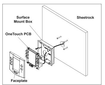
Figure 27. OneTouch™ Surface Mount Installation
