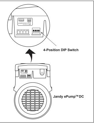
Figure 15. Jandy ePump<sup>™</sup> DC Dip Switch
