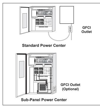
Figure 4. GFCI Installation for High Voltage Underwater Lighting
