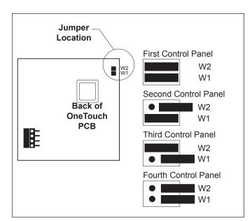
Figure 32. Jumper Settings for Multiple OneTouch™ Control Panels
