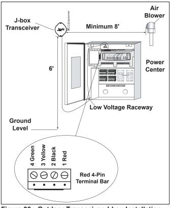
Figure 33. Outdoor Transceiver J-box Installation for Wireless OneTouch<sup>™</sup> Control Panel
