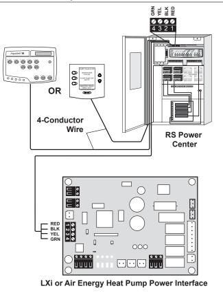
Figure 18. Jandy LXi<sup>™</sup> Heater and Air Energy Heat Pump Connection to Power Center
