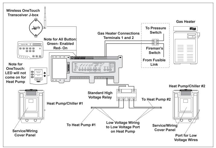
Figure 19. Heater and Heat Pump/Chiller Wiring
