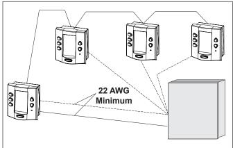
Figure 31. Installing Multiple OneTouch Control Panels
