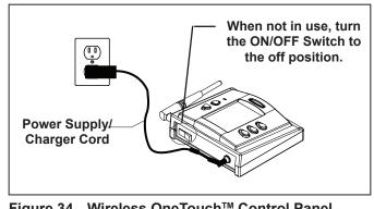
Figure 34. Wireless OneTouch™ Control Panel Installation
