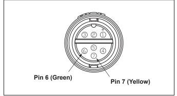
Figure 14. Cable Connector at the Pump Side
